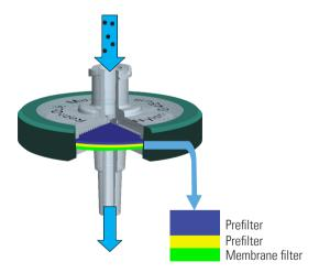
RephiQuik Max filters contain 3 filtration layers, which reduce blockage and increase volume throughput.
