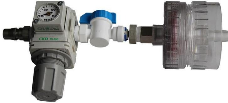
Silt Density Index (SDI) is a measurement of the fouling potential of suspended solids and colloidal to the RO membranes. A feed SDI reading of less than 5 is considered acceptable.
